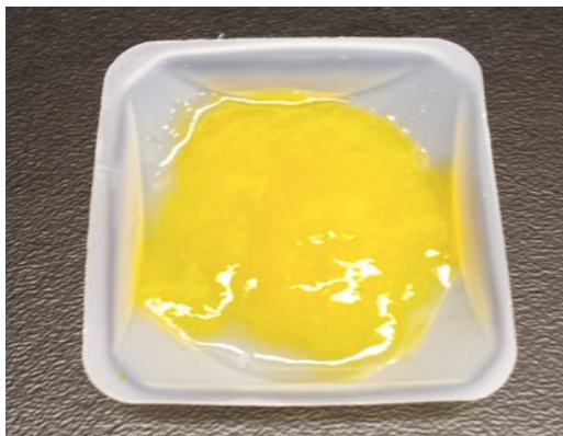
Figure 5.15: Image of wet bulk fibers loaded with curcumin with a visible yellow hue after washing to remove surface curcumin.
